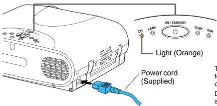
The three indicators, TEMP, LAMP, and ON, light in green for several seconds and then the ON indicator lights in orange and the projector turns to the standby mode.
